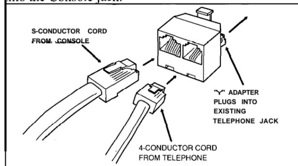
Figure 11. Telephone "Y" Adapter Connections
