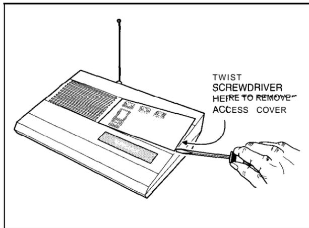
Figure 15. Removing Access Cover
