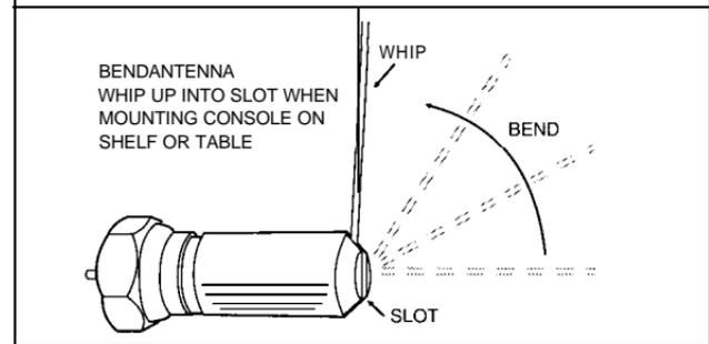
Figure 10. Bending Whip Antenna
