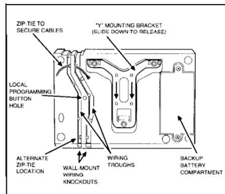
Figure 8. Console Base and "Y" Mounting
