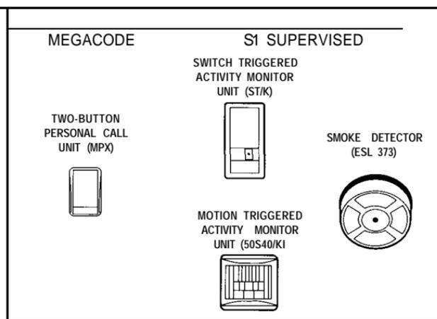
Figure 3. Typical Transmitters
