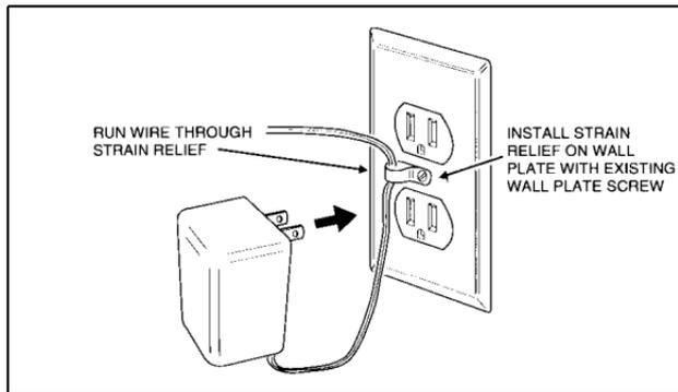
Figure 8A. AC Power Supply Installation
