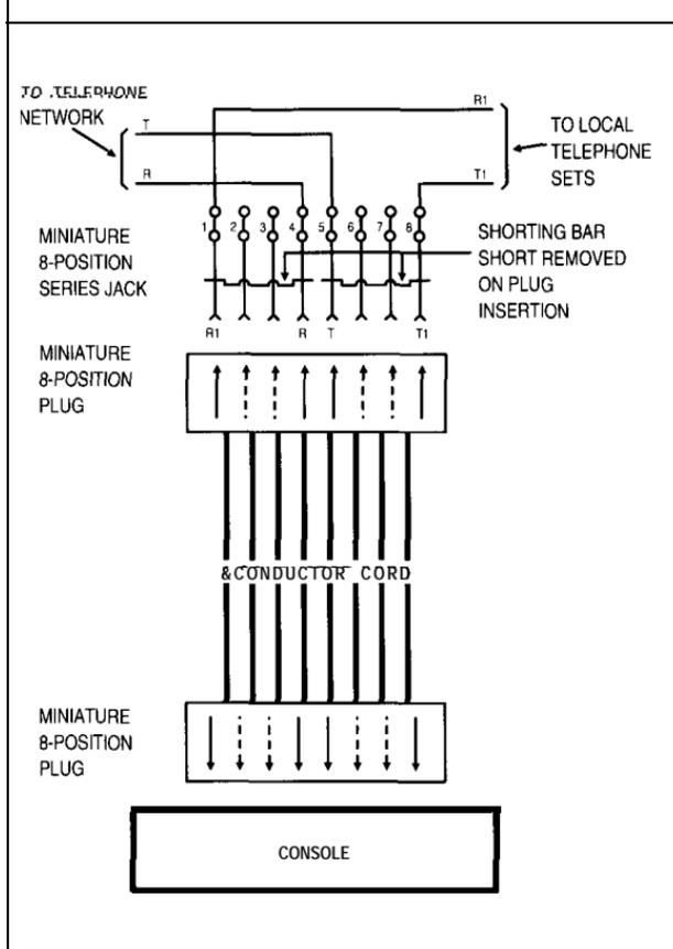
Figure 12 U.S.O.C. RJ31X Telephone Jack Wiring
