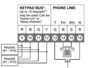
\* = Maximum wire length each: 1000 ft. (305 m). Maximum wire length total in system: 6000 ft. (1830 m) when using #22 AWG (0.8 mm) or #18 AWG (1.0 mm) cable.
