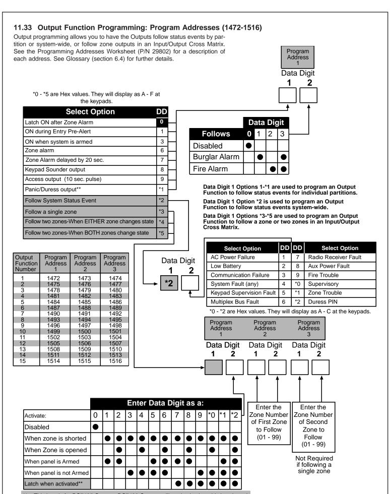
\*\* = This is only for DS7465 Outputs. DS7488 Outputs will not latch when this is selected.
