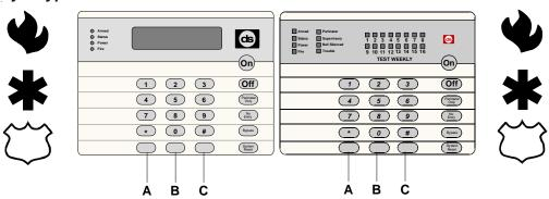
The Emergency Alarm Keys [A], [B], and [C] may generate Fire, Special Emergency, and Panic Alarms if programmed by the installer. Ask your installing company to explain the function of these keys.
