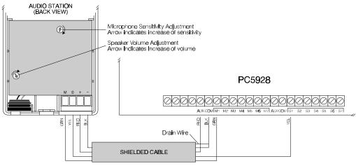
\* Connect drain wire to the COM terminal of PC5928 OR the black terminal of the station - NOT BOTH
