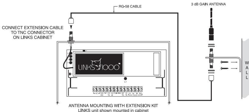
**Use only the Extension Kits to extend the mounting range of the antenna. Do not cut or splice the extension cable.** The maximum distance between the LINKS and the antenna is 25 feet (7.62 m) as obtained by using the LAE-25 Extension Kit. Make sure the antenna is in a physically secured location to avoid tampering.
