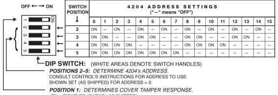
ON = DISABLED (SHOWN, AS SHIPPED) OFF = ENABLED (COVER IS TAMPER-PROTECTED)
