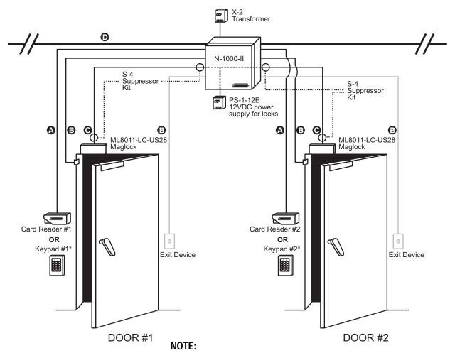
Door strikes (NS112S-R) or magnetic locks (ML8011-LC-US28) can be used to secure doors.
