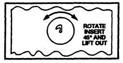
The connector may be installed in any of four positions. Install so that the antenna is vertical—either pointing up or down, not to the side, when the transmitter is mounted. Mount the connector using the 4 screws provided.
